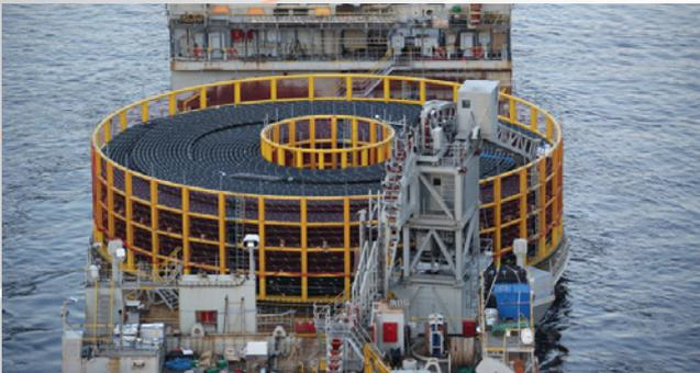
Working in partnership and developing the product with our client through design conception, we carried out simulated trials to ensure the assemblies performed to design specifications. The Assemblies we manufacture range from Roller Assemblies weighing 200Kgs to Central Hub Assemblies weighing 10000Kgs, the largest being for a 7000 tonne carousel.
